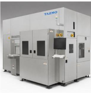
We develop, design, manufacture, and sell temporary bonding and debonding systems that enable wafer thinning, an essential process for the production of high-performance chips. By bonding wafers to glass carrier substrates, our systems allow wafer thinning while preventing damage to the wafers.
